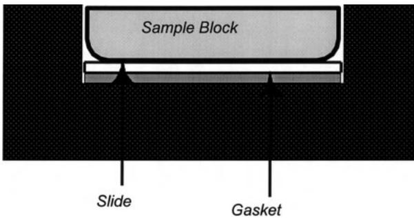
Fig. 4b. Compression of the sample block seals it to the slide, which is in turn supported by the gasket and carrier. The tops of the carrier and sample block have been removed
