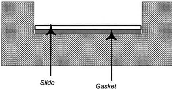
Fig. 4a. The gasket is first placed in the carrier followed by a cleaned slide
