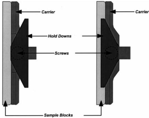
Fig. 4c. At the left, the hold down is shown rotated, which permits the sample block to be inserted or removed. At the right, the hold down is shown rotated 180°, which locks the sample block into place and seals the block to the slide
