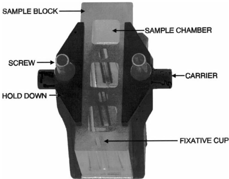
**Fig. 1.** Aluminum carrier version of the Centrifugal Cytology bucket. The carrier is supported by and pivots on the two cylindrical pins. Loosening of the two screws permits both of the hold downs to be rotated 180°. This permits insertion or removal of the sample block, microscope slide, and foam pad
